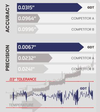
\*Calculated from 24 finger tool(s) average inner diameter reading through 350°F temperature drift @ 45″ soak periods @ 50°F steps.
